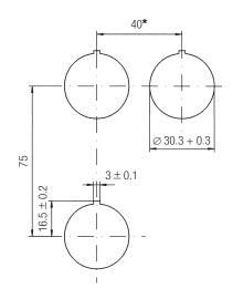
\* Recommended distance for mushroom pushbutton, emergency switch as well as position selector with protective shroud: 100 mm.
